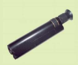
The Fiber Inspection Scope utilizes a white Light LED for co-axial illumination. Light is introduced into the optical path (axis) so that it passes through the objective lens and adapter tip striking the ferrule perpendicular to the end face. This method of illumination produces a high level of resolution providing excellent detail of scratches and contamination.
